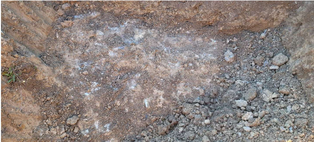
Picture 11: TH-04 - Close up view of bedrock surface.
